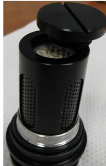
Figure 1: New Desiccant (Left) and Slotted Cap Removed (Right)
